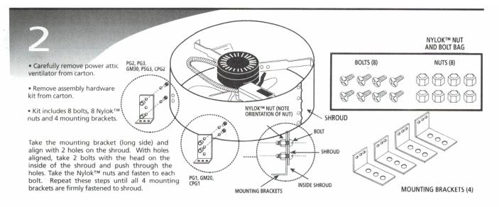
Place mounting brackets so end is flush with stud. Mount on gable end, behind existing louvers (Fig. 3 or 4), or install behind MASTERFLOW™ Automatic Gable Shutter, part number SGM20 (sold separately).
