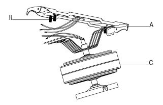
Once wiring is completed, lift the motor bracket on the top of the fan-motor assembly (C) so that the threaded studs (II) on the mounting plate (A) protrude through the slot in the motor bracket. Securely tighten the three locknuts (BB) onto the threaded studs (II), then try to shake the fan-motor assembly (C) to ensure that the assembly is tight.
