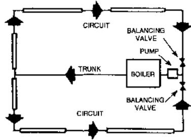
**3. ONE PIPE WITH DIVERTER TEES** Permits individual room shut-off or thermostatic control. Each baseboard unit is connected to the main by a supply and return branch connection (usually with a shut-off valve at the diverter tee). This offers a sophisticated system of room temperature control, particularly in conjunction with Slant/Fin's fully modulating damper.
