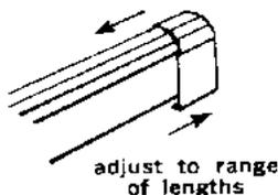
Slant/Fin baseboard units come in a wide variety of standard lengths. The Slant/Fin accessories simply snap over and behind the baseboard units permitting them to slide left or right. The amount of overlap can be adjusted from only 1/2" to almost the full width of the accessory. This way you can virtually "stretch" or compress standard lengths of baseboard and accessories to fit any length of wall without cutting them. Slant/Fin installs faster than any other baseboard in the world.
