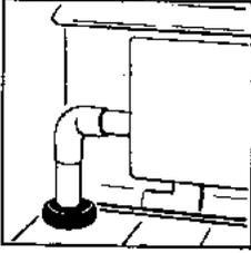
**RISER-RINGS** slip around tubing where it passes through flooring. They provide neat, clean, sanitary seal and absorb expansion squeaks and vibration noises. May be installed after connections are made.
