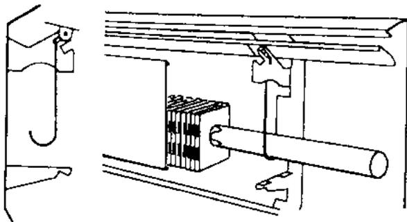
Use Slant/Fin hanger to support the bare tubing at the same height as adjoining heating elements. Insert the short hook of the hanger as shown. Install from the left side, so that the large hook (which holds the tubing) faces the rear panel.
