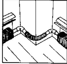
**PEX-TO-BASEBOARD CONNECTOR** When PEX tubing is used to and from the boiler, Slant/Fin Terra Therma PEX adapters connect tubing to copper baseboard heating element.
