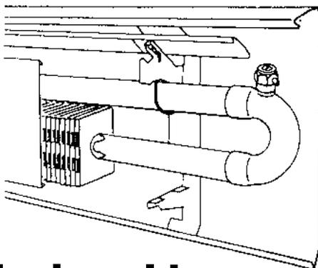
Note: If the baseboard is installed below the boiler level, as in many slab jobs, the return bend may be installed with the vent opening pointed downward, and plugged. This permits easy drainage if needed.
