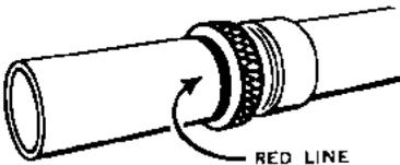
**PULL OPEN** until red line just shows under the knurled collar. Install in this extended position.
