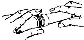
**DON'T LOOSEN** or tighten the knurled collar. Proper adjustment (set at factory) is hand-tight only.
