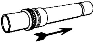
**FLOW DIRECTION** must be as shown, to keep sludge from clogging the seals inside the Hydro/Tite.
