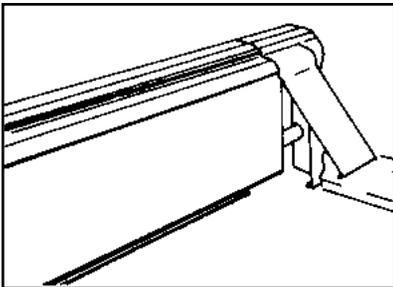
For a neat finish at partitions, use the wall trim (adjustable up to  $3\frac{1}{2}$ " ). Air vents are recommended at each drop; either wall trim or end caps (both hinged) provide easy access to vent. These accessories eliminate the wasteful need for cutting large baseboard units to fit small gaps, and save you time and effort. Attractive inside and outside corners assure a custom look.
