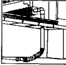
**FAST/FLEX CONNECTORS** can be hand-formed to fit varied piping problems. Use them to fit around obstructions, compensate for misalignment, soak up vibration and expansion at turns, eliminate many solder joints. Cannot be used as an expansion compensator.
