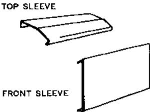
1. When mounting the baseboard to the wall, be sure the filler sleeve will overlap each baseboard unit by at least 1/2".
