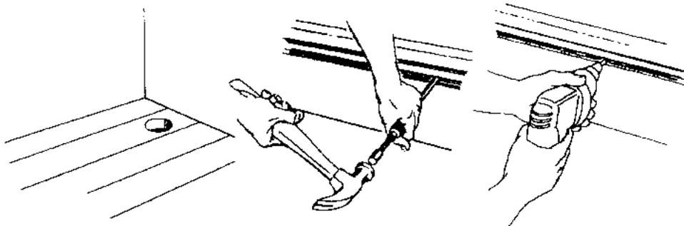
**1.** Drill holes for risers and connecting piping.
