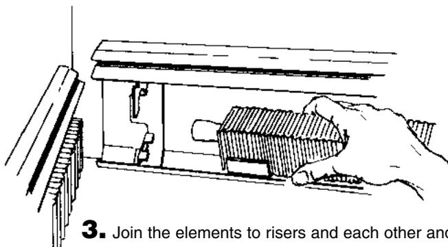
**3.** Join the elements to risers and each other and rest on brackets.
