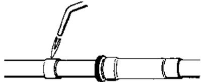
**KEEP HEAT AWAY** from the knurled collar and the coupling body, to avoid damage. Use soft solder only.
