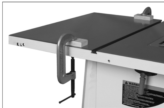
Figure 6-6: leveling extension wings, method 2
