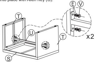
**Note:** If any screw holes cannot be aligned, pls loosen all the screws and go back step 1 and restart assembly.
