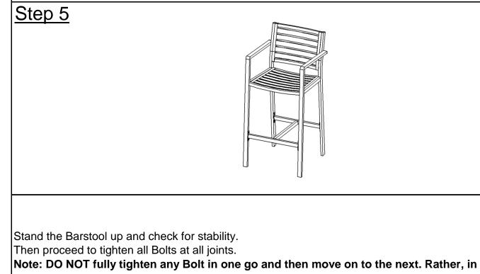
a sequential manner, gradually tighten each Bolt until all Bolts are evenly secured. This methodology will ensure maximum evenness once all Bolts are fully tightened. Your Barstool is ready for use.
