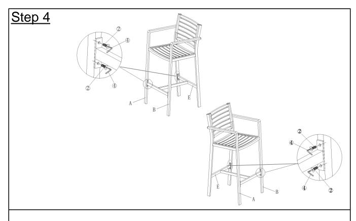
Attach Footrest(E) between Right Leg(B) and Left Leg(A) using Bolts(2) with Allen Key(4) as shown above.
