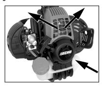
Removal of cooling passage blockages or cleaning of cooling fins is considered "Normal Maintenance." Any failure attributed to lack of maintenance is not warranted.
