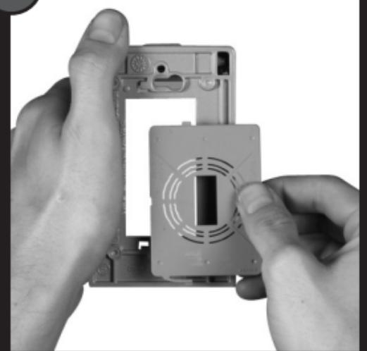
Configure adapter then snap it to the back of base.
