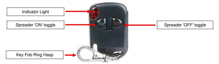
The spreader has been supplied with two remote key fobs, and one remote receiver, factory installed in the spreader unit. Both supplied key fobs are already paired specifically to the receiver, so there is no need to perform any pairing with the system. Care has been taken when packaging the spreader unit to keep the specific remotes together with the properly paired receiver.
