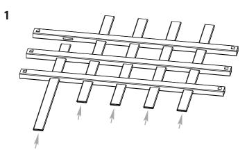
3 NOTE: There are locking tabs located at the ends of the horizontal rails. Once inserted and pushed into the routed holes, they will lock into place.
