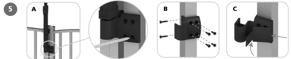
**A:** Position the striker with the bottom of the latch and mark the location of the mounting holes on the gate.
