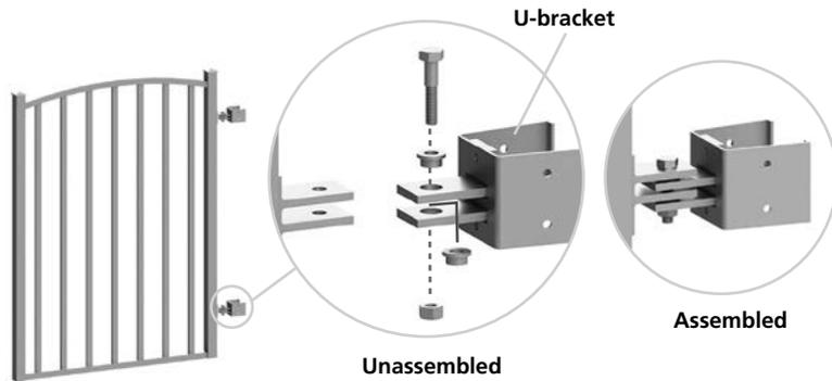
Install each hinge and U-bracket assembly on the gate and secure with bolt, bushings and nut (provided).
