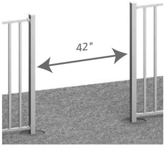
The opening between the fence posts must be 42".
