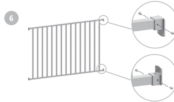
Install a bracket on each end of both rails and fasten in place with 5/8" self-drilling screws (provided). Ensure the tabs are facing towards the center of the fence panel.
