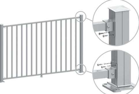
Attach the fence panel to the posts using 5/8" self-drilling screws (provided).
