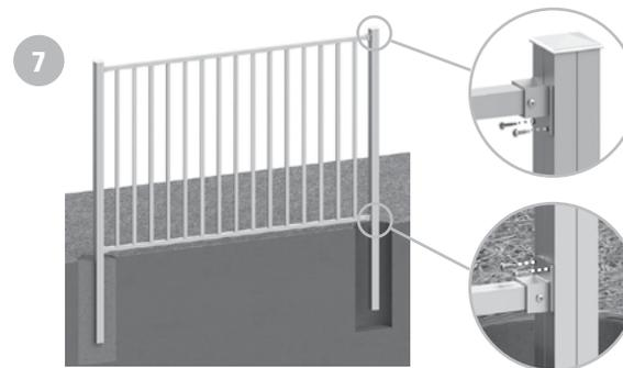
Attach the fence panel to the posts using 5/8" self-drilling screws (provided).
