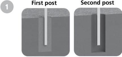
Measure and mark the position of all posts and ensure they are aligned. Dig the post holes.
