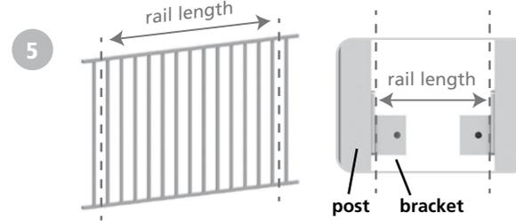
**If required,** cut the rails to fit between the brackets.
