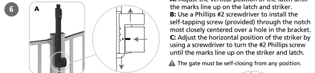
**A:** Adjust the vertical position of the latch until the marks line up on the latch and striker.
