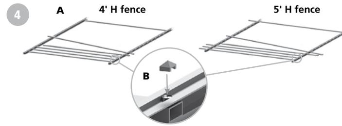
**A:** Install all remaining pickets and fasten the pickets to the rails using 1/2" self-drilling screws and washers (provided).
