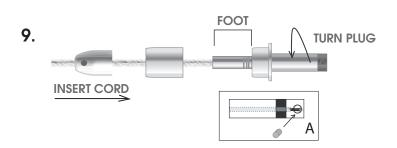
Reassemble the Quick Adapt connector by passing the cord through the retainer and sleeve first. Then insert the cord into the turn plug making sure that the foot of the plug covers the braided jacket. Turn the plug while inserting the cord for an easier insertion. Make certain you can see the center wire at the top opening A of the plug to ensure a good connection.
