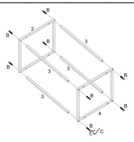
Attach part (2,4) to part (3) using bolt (B) with hex key (C).
