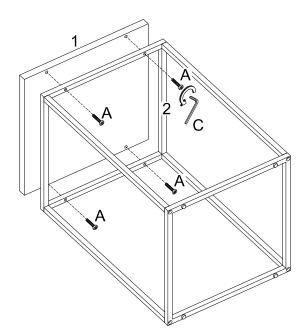
Attach part (2) to part (1) using bolt (A) with hex key (C).
