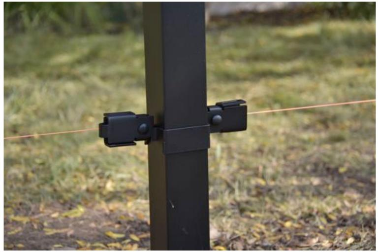
Middle Brackets will have two short carriage bolts and grip nuts to hold the bracket onto the post temporarily until the Stringer has been placed on and leveled.
