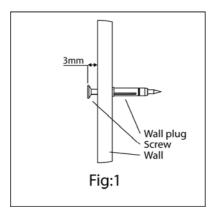
5. Align the keyhole fixings on the rear of the product (see Fig 2) with the protruding screws and push down firmly to ensure the product locates tightly against the wall. If adjustment is required remove the product and either loosen or tighten the screws until the product is held firmly in place.
