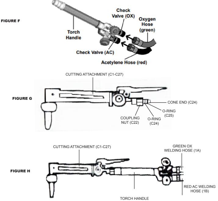
**6.** Check connections for leaks. Adjust the acetylene regulator (parts 1-19) and oxygen regulator (parts A1-A20E) to their normal operating pressure. Use an approved leak detection solution to check for leaks at the welding hoses (A1 and 1B) and cylinder valve connections. If leaks are fond, tighten nuts more securely.
