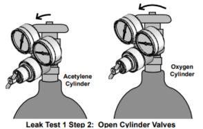
**3.** Open the Oxygen cylinder valve completely, turning it counter-clockwise.
