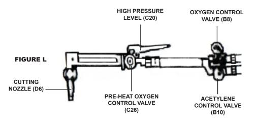
**12.** Open the acetylene control valve (B8 with AC label (B10) on the torch handle. Adjust the acetylene regulator (parts 1-19) to the desired working pressure. Then close the acetylene control valve on the torch handle. See figures E and L
