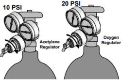
Leak Test 1 Step 4: Set Testing Pressures
