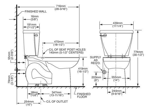
NOTES: THIS TOILET IS DESIGNED TO ROUGH-IN AT A MINIMUM DIMENSION OF 254MM (10") FROM FINISHED WALL TO C/L OF OUTLET. SUPPLY NOT INCLUDED WITH FIXTURE AND MUST BE ORDERED SEPARATELY. \* DIMENSION SHOWN FOR LOCATION OF SUPPLY IS SUGGESTED.
