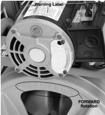
Figure 8 – Proper Drum Rotation (FOR Switch Position)
