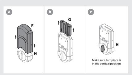
B Install 4 AA batteries in battery pack.
