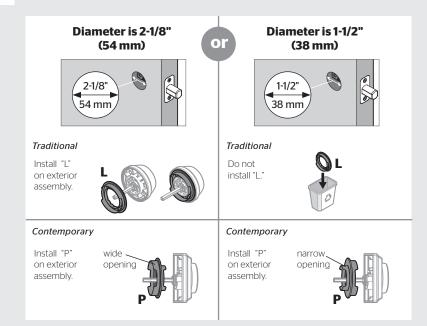
C Install exterior assembly and mounting plate.
