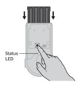
3 Press the Program button once more. When the LED flashes green and you hear two beeps, the lock has been reset.
