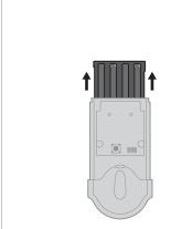
2 Press and HOLD the Program button while reinserting the battery pack.
