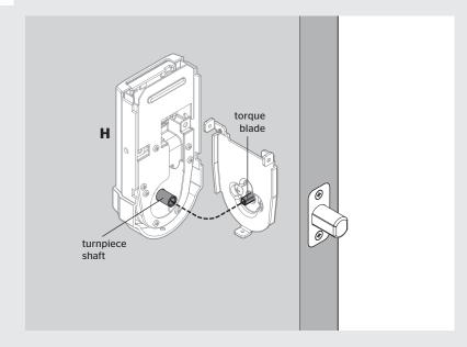
Secure interior assembly with supplied screws.
