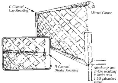
the cap at the bottom of the groove. Plan on using approximately 1" of extra moulding material for each miter joint you make.
