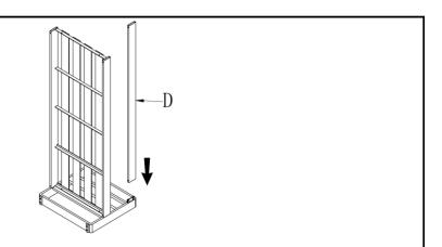
Insert the Back Support Bar(D) into the Left Side Panel(A).
