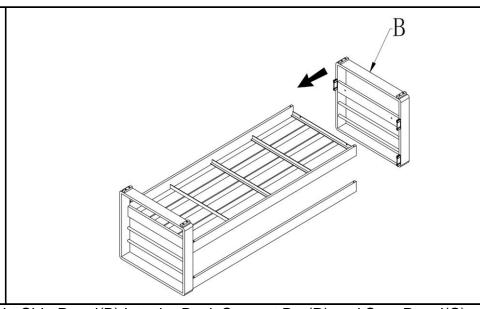
Insert the Right Side Panel(B) into the Back Support Bar(D) and Seat Panel(C) as shown above.
