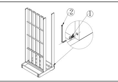
Attach Back Support Bar(D) to the Side Panel(A) using Bolt(1) with Allen Key(2). **Do not fully tighten the Bolt.**
