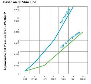
Flow Rate - gpm (lpm)\*
