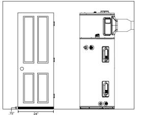
Heater: Ducted with inlet AND outlet duct
