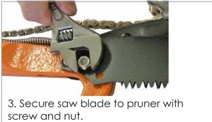
3. Secure saw blade to pruner with screw and nut.
