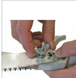
Replace lock washer and wing nut, tighten.
