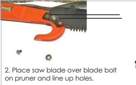
2. Place saw blade over blade bolt on pruner and line up holes.
