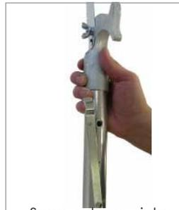
Snap pole saw into pole's ferrule.
