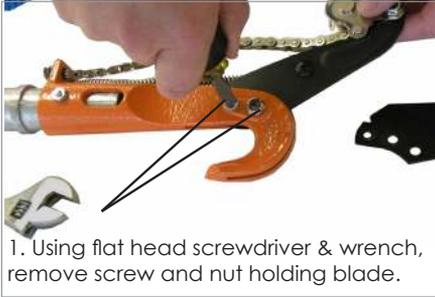
1. Using flat head screwdriver & wrench, remove screw and nut holding blade.
