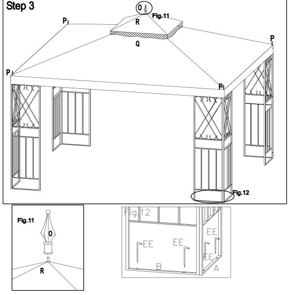
**Fig.11:** Put Small Canopy (R) to small top, put Centre Finial (O) to small top connector. Put fully spread Big Canopy (Q) to the big top, screw Corner Finial (P) into four corner on the big top.
