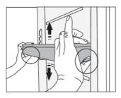
The height of the door bins/shelves can be adjusted to your preferences without having to take them out of the appliance. Gently squeeze the tabs on both sides and move the bin/shelf up or down. To remove a bin from the appliance, lift it as far as it will go and pull it out.
