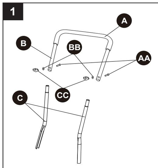
2. Attach the top handle subassembly to the lower handle (D) using four carriage bolts (AA), washers (BB), and fixing knobs (CC).
