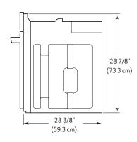
The first step of the installation is measure the current cutout dimensions and compare them to the cutout dimensions shown below. Little or no cabinet work may be necessary.
