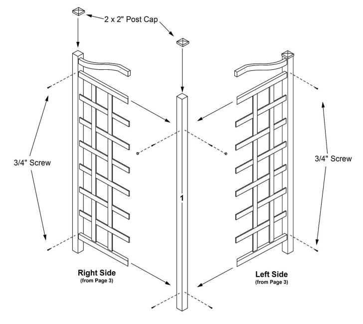
Insert left and right trellis panels (from Page 3) into 65" corner post (part 1). In order for trellis to look symmetrical, top/bottom cross rails, horizontal slats and bent tops must be fully inserted into 59½" left and right posts. Using two ¾" screws per outer post and four ¾" screws for corner post, fasten together trellis. Using PVC, super or crazy glue, apply glue to inner corners of each 2" sq. post cap and place on top of each post.
