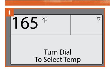
After turning ON (I) the Main Power switch, your grill's home screen defaults to the "Turn Dial To Select Temp" message. Cooking temperature can be set directly from this screen.
