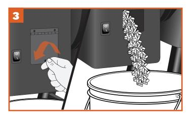
Unscrew the clean-out door fastener and open it. Pellets will empty into the container you've placed below. You might need a spatula or spoon to push the remaining pellets out of the hopper.
