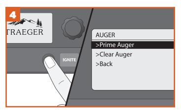
Press MENU to display the main menu. Turn the dial to select AUGER, then select Prime Auger.
