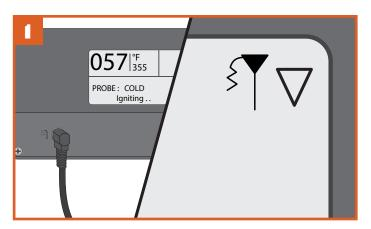
Plug the probe into the probe jack located on the WiFIRE Controller. See "Using Your Grill" to turn on the grill. Once the grill is on, the controller will recognize the probe and the probe icon will light in the controller screen's upperright corner.
