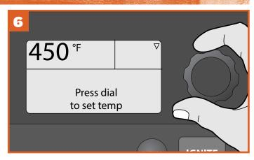
After completing Step 5, adjust temperature to 450°F (232°C) and run grill for an additional 30 minutes.
