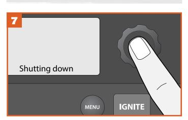
Turn off the grill by pressing and holding the Selection dial for 3 seconds, initiating the shutdown cycle. When the full shutdown cycle finishes, seasoning of your grill is complete.
