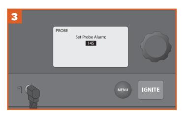
Rotate the dial to the desired food temperature. Press the dial center to select/confirm.
