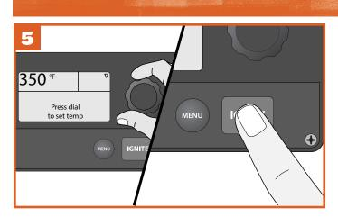
The home screen will display "Press dial to set temp." Turn the Selection dial clockwise to 350°F (I77°C) and press the dial. Next, press IGNITE, close grill door, and run grill for 20 minutes once it has reached the set temperature.
