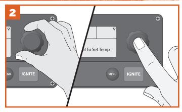
To select temperature, turn Selection dial right or left; once desired temperature is displayed, press the center of the dial to select.
