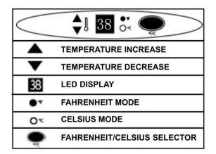
When you first plug in your Kegco refrigerator, the LED display will show the "live" cabinet temperature in Fahrenheit and the thermostat will be set to 41 degrees Fahrenheit (5 degrees Celsius). The operating panel includes several other features to operate and control the temperature of the refrigerator:
