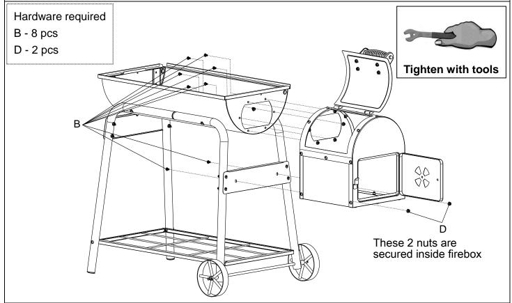
Step 8. Attach firebox lid stopper (#31) to firebox using 2 pcs of bolts M6 x 12 (B) and 2 pcs of flange nuts M6 (D). Attach Firebox door vent (#32) and firebox door lock (#33) using 2 pcs of bolts M6 x 12 (B) and 2 pcs of lock nuts M6 (F) and 1pc of washer (H). <u>Tighten</u> bolts and nuts <u>with tools</u> in this step.
