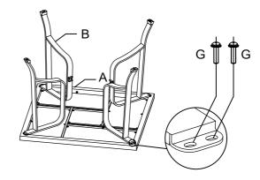
Place table top frame (A) on the ground, then screw table legs (B) to it. Please do not tighten any screws to the end at this step.
