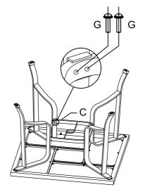
Screw table leg support ring (C) to table legs. Make sure all screws are inserted properly and tighten all screws to the end.
