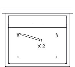
For brick or other masonry wall, insert a plastic anchor (included) into each hole. Tap in gently if necessary. This step is not required if mounting on a wood wall.
