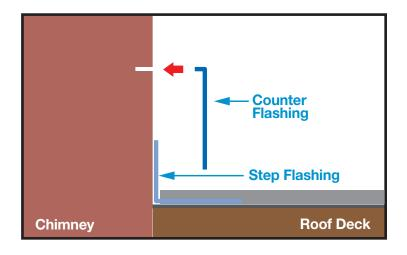
Galvanized counter flashing has sharp edges. Use gloves to prevent injury. This product is not recommended for direct contact with treated lumber.
