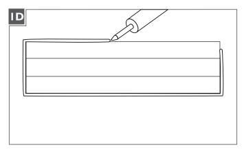
For wet locations, caulk around the base with waterproof construction sealant.
