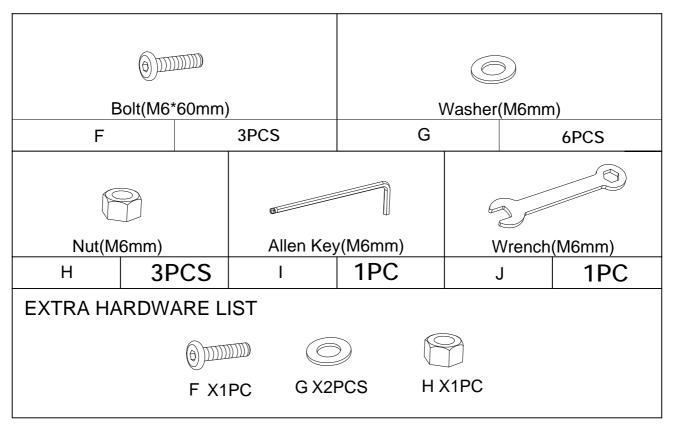
Step 1. Attach Right Seat (B) to Left Seat (A) using the Bolts(F), Nuts(H), Washers(G), Wrench(J) & Allen Key (I).
