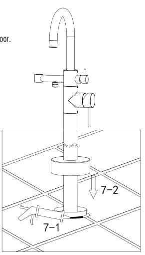
**8** Connect the hose and the hand shower ,then rest the hand shower in the holder. Turn on on-off valve to test the situation of water.
