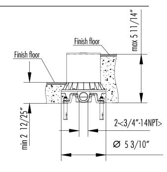
Put the embedded part into the hole,draw the location of the mounting holes. Make sure that the level of location of embedded with spirit level . Then remove the embedded part ,drilling with  $\varnothing 2/5$ " drill and put the setscrew in the mounting holes and place the embedded part on the setscrew, tighten the screws with a adjustable wrench.
