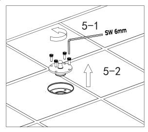
**6** Get the faucet from the packing and push up the escutcheon. Connecting the faucet with the embedded part . Then adjust the direction of faucet and tighten the screws using an 6 mm Allen wrench.
