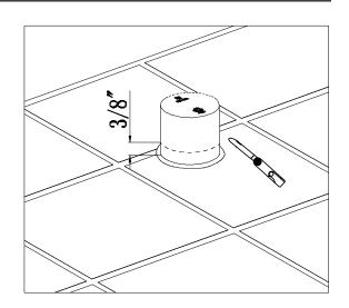
**5** Loosen the lock screws, set aside. Then remove the sealing test plug.
