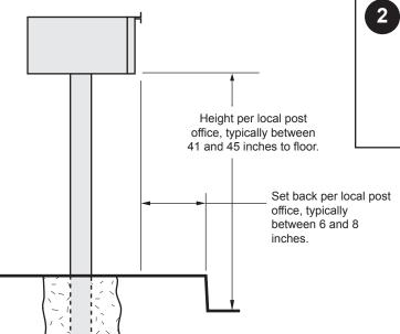
For 3" Round In-ground Post (item 7507, 7510, 7511, 7513, or 7516) or Standard In-ground Post (item 5525): Pour the concrete (at least 1 cubic foot recommended) completely around the post, making sure the post and mailbox are level and correctly positioned according to your local post office.
