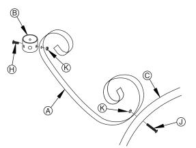
Typical assembly for SCROLL (A), SUPPORT RING (B), CURVED CONNECT BAR (C) using SCREW SHORT (H), SCREW LONG (J) and HEX NUT (K).
