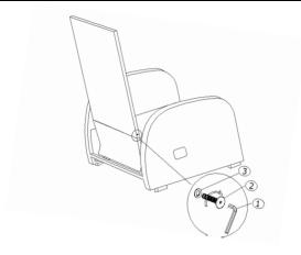
Attach the Chair Back(C) to Chair Base(A) using Bolts(②) and Washers(③) with Allen Key(①) as shown in the picture above.
