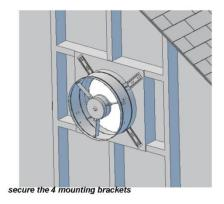
TIP: Much of the preparation, wiring of thermostat, testing, and mounting to the frame can be done before final installation in the attic.
