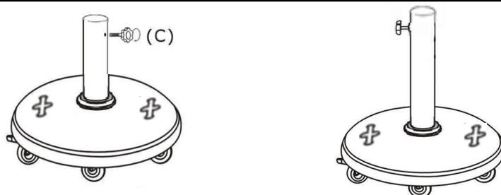
Screw Adjustable Screw(C) into Support Pole(B).
