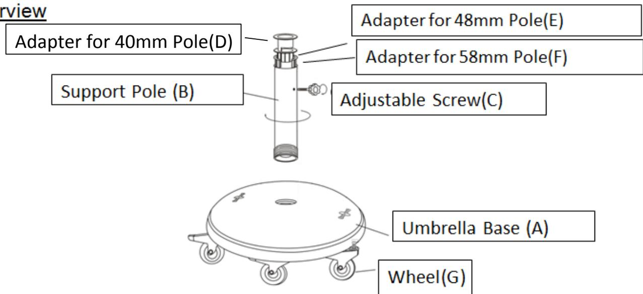
This Umbrella Base has multiple parts and may require up to 30 minutes to assemble. To give you an overview of the Umbrella Base parts, the above picture is to help you put the various parts into perspective. Please read through the instructions below to familiarise yourself with the parts and steps before assembly.
