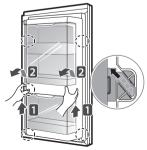
2 To replace the Door-In-Door case, line up the tabs on the Door-In-Door Case with the slots on the door and push the case down until it snaps into place.
