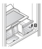
To install, slightly tilt up the front, insert the drawer into the frame and push it back into place.
