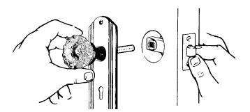
truding spindle and screw the remaining knob onto the spindle, snugly to hold plates in place.
