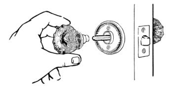
Loosen set screws and remove both doorknobs from the spindle. Center the spindle in door latch. Slide the threaded backplate over the spindle on the outside (most visible) side of the door. Slide its mate
