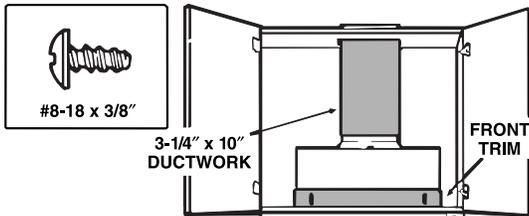
Complete the ductwork from the hood to the outside using a roof cap or elbow and wall cap. Tape all joints. Shelves may be installed if trimmed to clear the ductwork.
