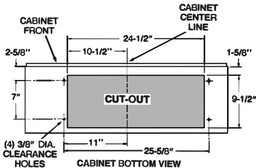
Prepare the cabinet bottom as shown above. Be sure to locate the cut-out and four holes from the front of the cabinet to assure a flush mount.
