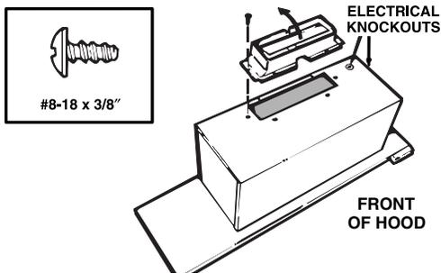
Use two (2) screws (provided) to attach the connector to the housing. The damper flap should open in the direction indicated by the arrow.
