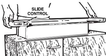
Carefully lower the housing into the cabinet opening with the slide control to the front.
