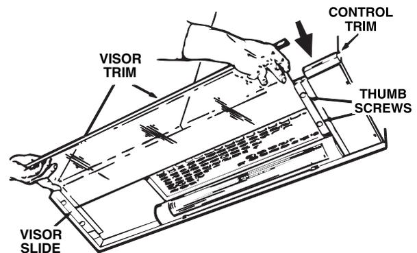
Slide the glass into the visor slides, above each visor clamp (see the illustration in step 14). Align the visor trim and tighten the thumb screws to secure the glass.
