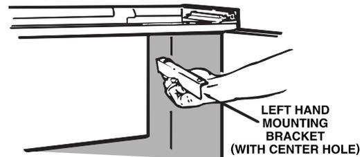
Hold the left hand mounting bracket in place on the side of the housing as shown.
