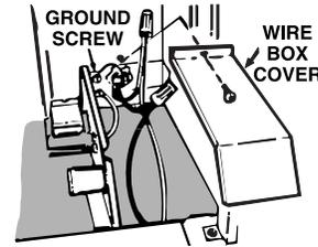
Remove the wire box cover. Attach the power cable to the hood using the proper connector. Connect black to black, white to white and green or bare wire to ground screw. Replace the wire box cover.
