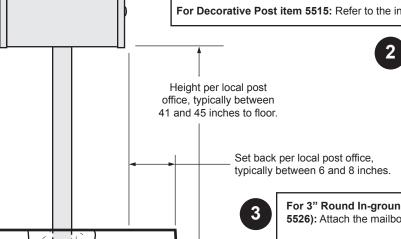
For 3" Round In-ground Post (item 7505 or 7507) or Standard In-ground Post (item 5525): Pour the concrete (at least 1 cubic foot recommended) completely around the post. making sure the post and mailbox are level and correctly positioned according to your local post office.
