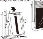
2. Pull out the Carbon Pre-filter and the HEPA Filter by grasping the tabs located on each side
