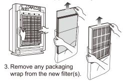
Place the new filters in the main unit. (HEPA filter should always be inserted first, then
