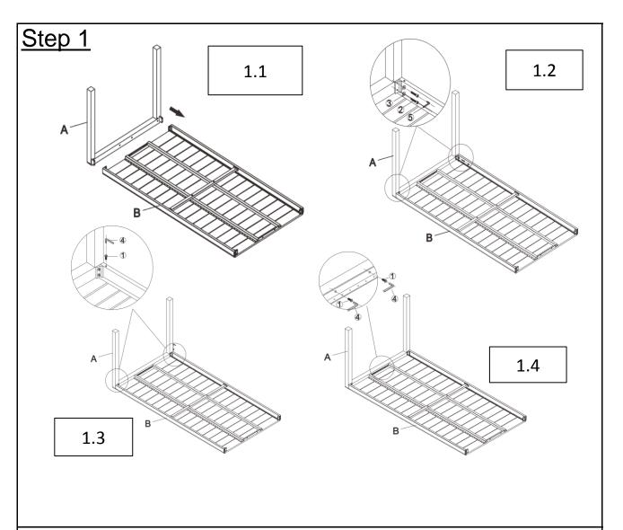
Open the carton and place all the parts onto a clean, non-marring surface. Place the Table Top(B) facedown.
