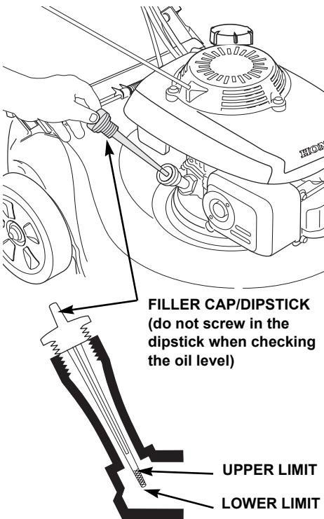
**Do not overfill engine with oil.** If the engine is overfilled, the excess oil may get transferred to the air cleaner housing and air filter.
